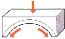
**Arch** - In the arch type of bridge, weight is carried outward along two paths, curving toward the ground.
