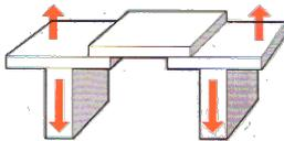
**Cantilever** - In the cantilever type of bridge, two beams support another beam, which is where the deck or trafficway is. The two beams must be anchored, and this must be done well.
